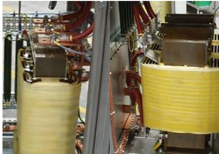
Figure 86. Entrance reactance, 'Main Choke', and the reactance of the current output of the rotor, dv/dt (Source: GDES-COMSA).
