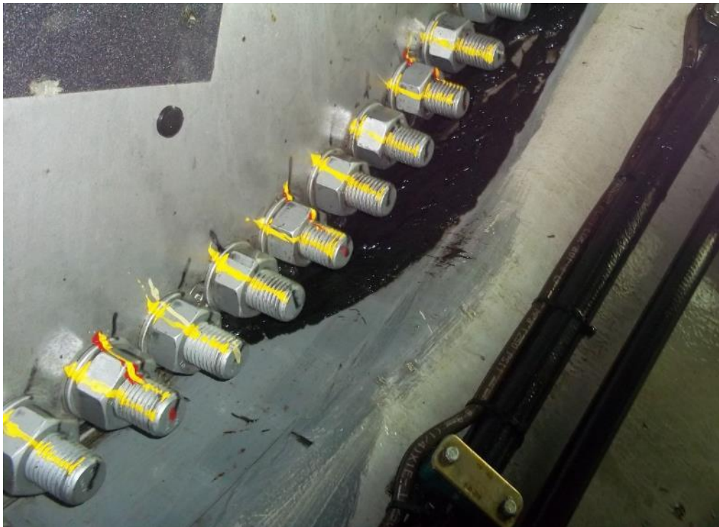
Figure 32. Blade Bearing joint bolts with torque marks
