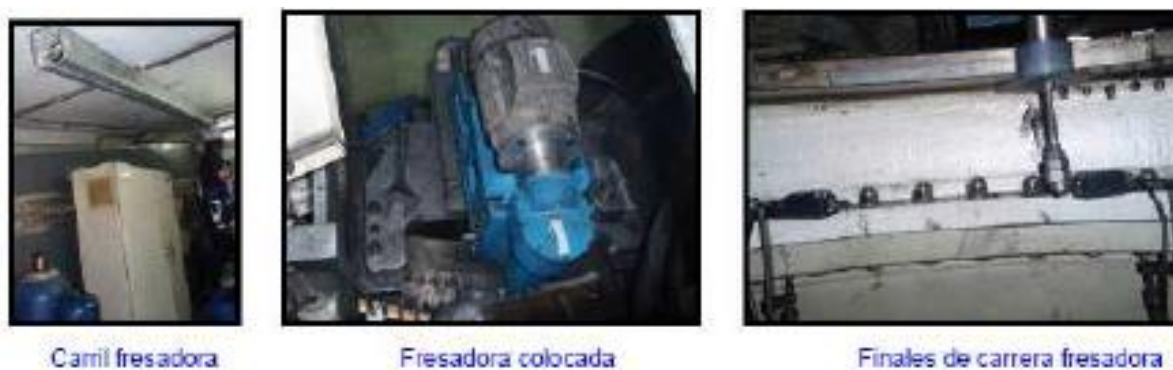
Figure 69. Placing the router to mill the damaged parts
