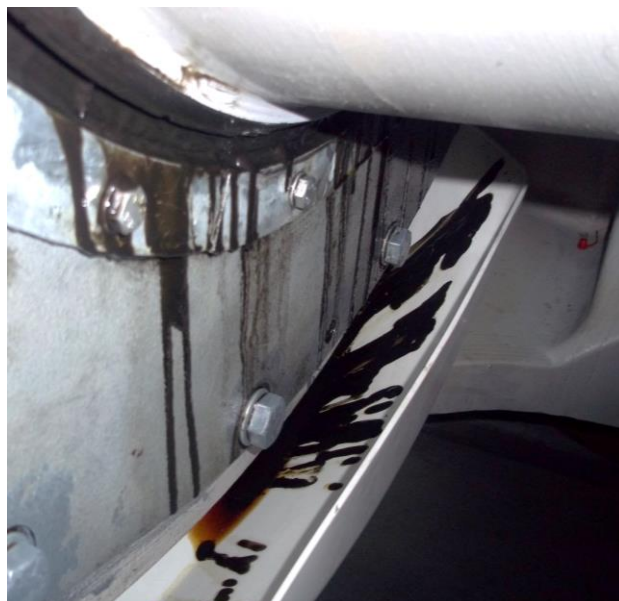
Figure 29. Grease leaking out of the bearing
