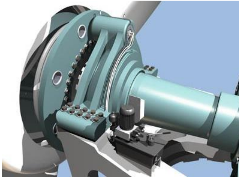
Figure 21. Locking pin connecting shaft and hub
